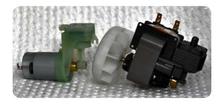
The photograph above shows a pump from a cheap machine on the left and a pump from a Lava machine on the right. The pump on the left is based on a generic motor which is made in China and weights 270 grams. The Lava pump is made in Germany especially for Landig and weighs over 1200 grams.
